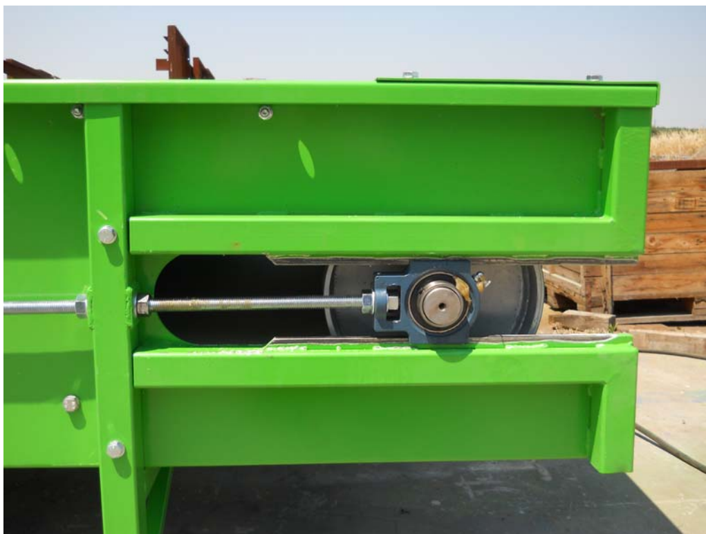
Figure 12 - Bearing support of idle roller
